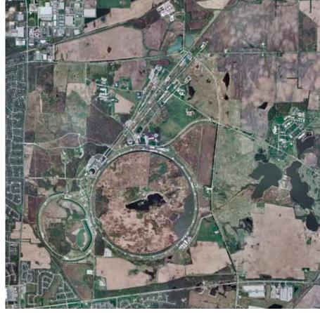
Ready, aim: The Tevatron (central ring) is going dark, but physics continues at Fermilab. Scientists are generating neutrinos using the smaller injector ring (lower left) and beaming them through the earth to an underground detector in Soudan, Minn., 450 miles away.
